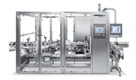
**CPS 0600** integration kit, here integrated into 3rd party bottle labelling machine including helper code application on the bottom/cap
