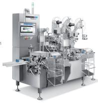
CPA 410 station for manual case aggregation by autofocus layer reading system, expandable with manual pallet aggregation
